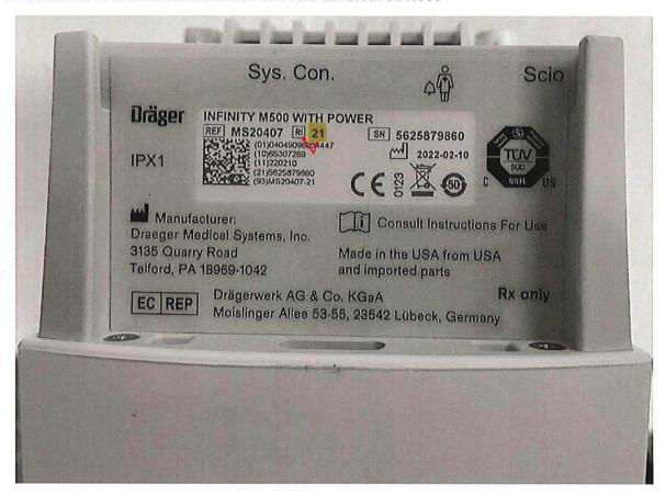
Red Arrow in picture above identifies revision (RI) of the device (MS20407 – Infinity M500 Docking Station). This label can be found on the underside of the device.
